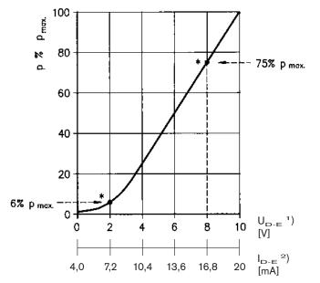
\* Factory setting at Q = 1 l/min  $\pm 5\%$  manufacturing tolerance
